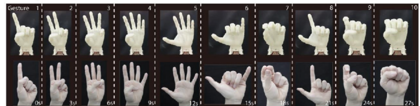
Gestures produced by the prosthetic compared to a human hand, both showing numbers 1-10 in Chinese sign language.
